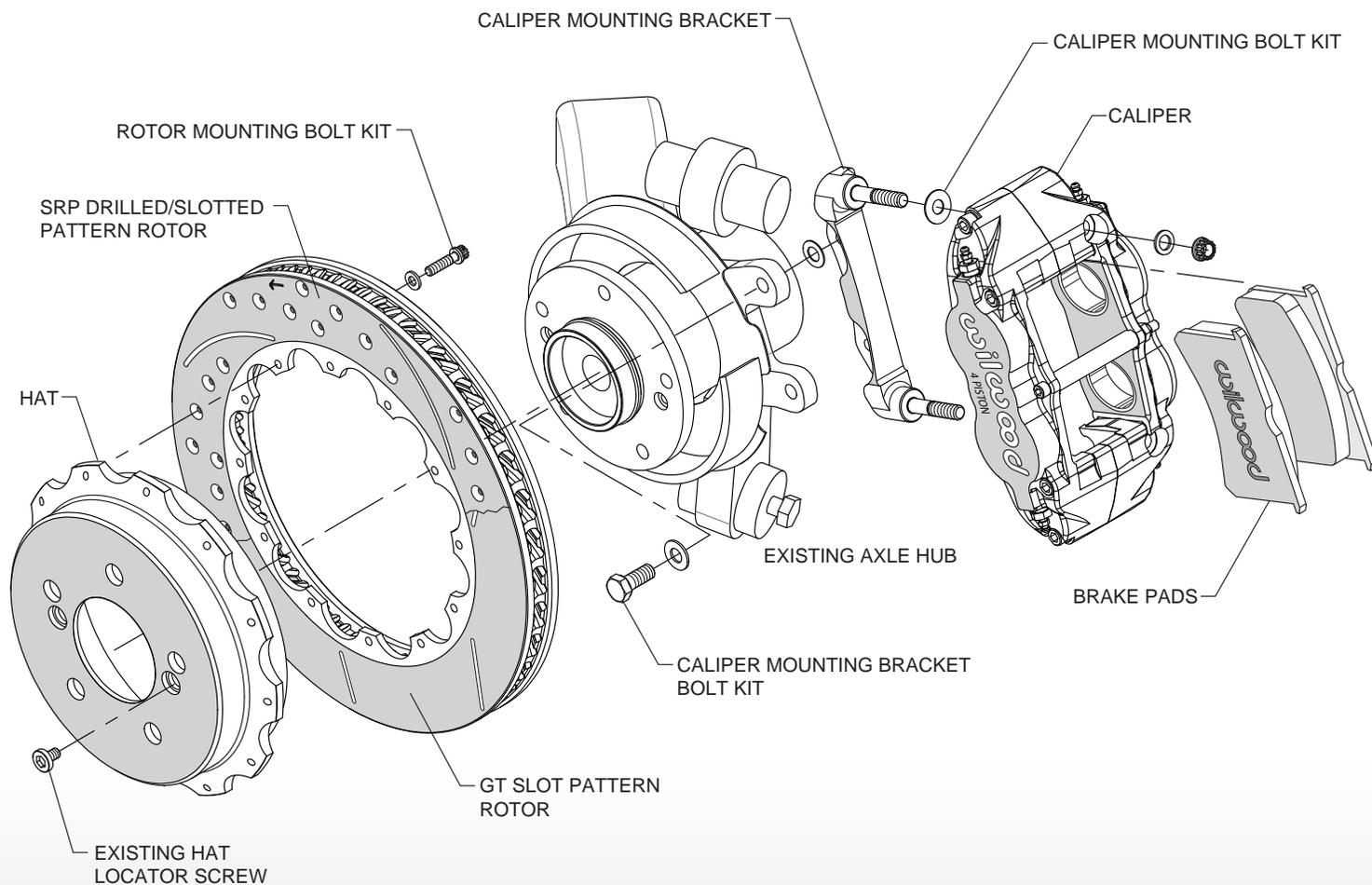
Figure 1. Typical Installation Diagram
